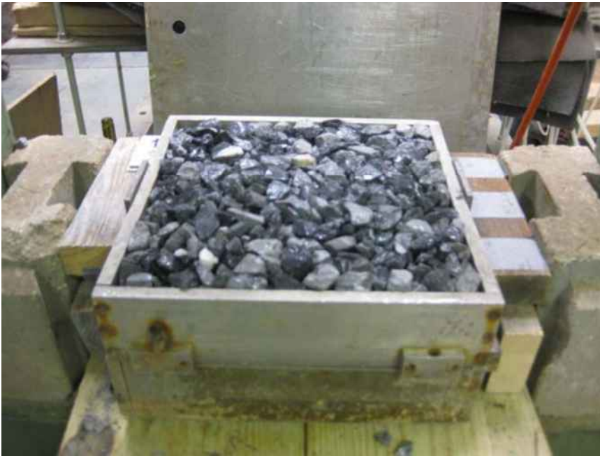
Figure 2. Compacted VDOT #57 stone in the lower box.
